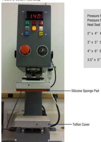
Pressure Settings Depending on Platen Size. Pressure Settings based on Texas Automation Heat Seal Machines with a 3" Cylinder.
